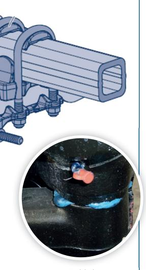
its steering pivot while the grease is applied so the cams ride over each other. The application should continue until fresh grease appears between the washers. Ideally, you'd have the trailer over a pit."
